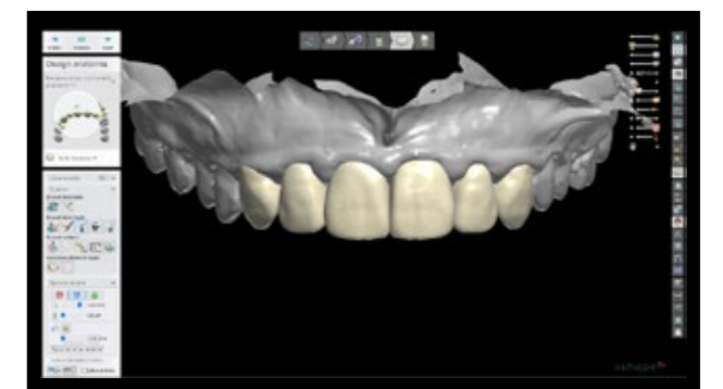
FIG. 5B Digital model of the maxilla in the CAD software with full-contour veneers designed for the incisors and canines according to the ideal shapes planned with digital smile design.
