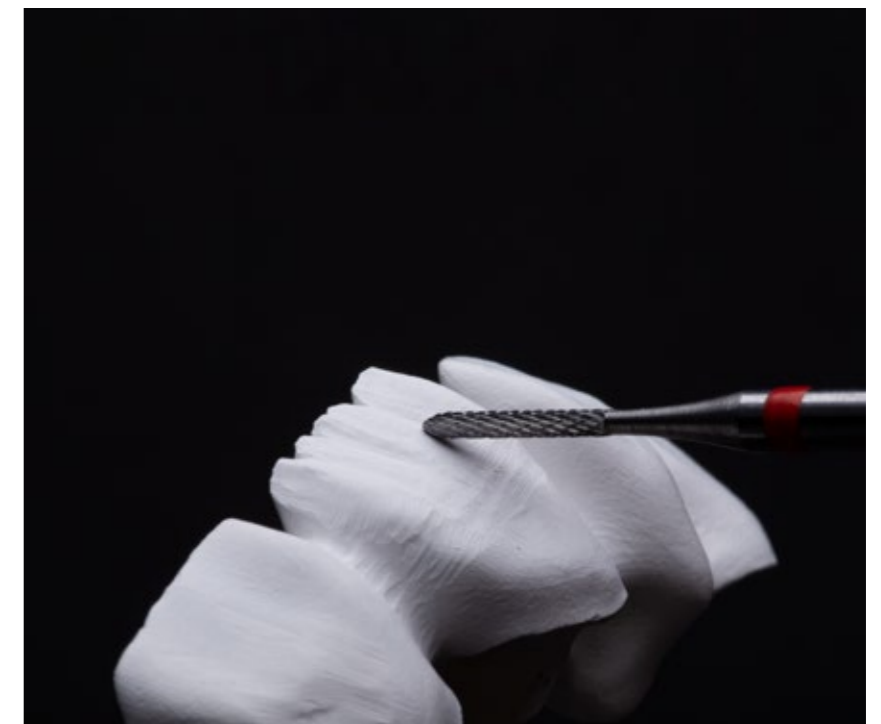
FIG. 06 Vestibular and incisal reduction and surface texturing on the pre-sintered restorations made of KATANA™ Zirconia.
